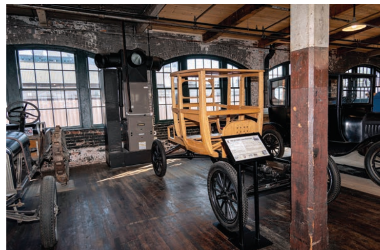
The 1919-1922 Model T Coupe Wood Frame at Ford Piquette Avenue Plant Museum. | CYDNI ELLEDGE / CRAIN'S DETROIT BUSINESS
